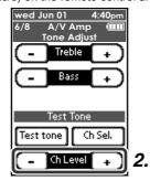
Adjust the speaker output levels so that you can hear the same sound level from each speaker at the listening position. For the front left, front right, center, surround left, surround right and surround back speakers, the output levels can be adjusted between –12 to +12 dB. The subwoofer can be adjusted between –18
